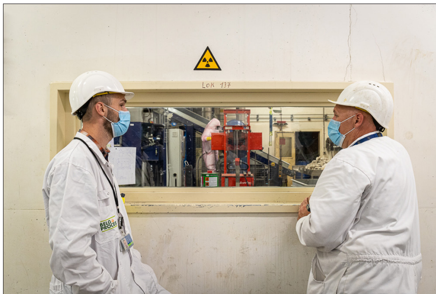
Figure 2. A look into a hands-on hot cell, where manual interventions and handling of radioactive contaminated materials can be carried out in safe working conditions
