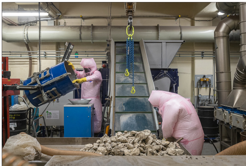
Figure 5. Pilot installation at Belgoprocess dealing with characterisation of concrete containing radioactive waste materials—sorting table and conveyor to shredder (front) and rotary sampler addressing more granulated drum content (left). This pilot experiment equipment setup can easily be scaled up by incorporating industrialised versions of, for example, rotary sample dividers.
