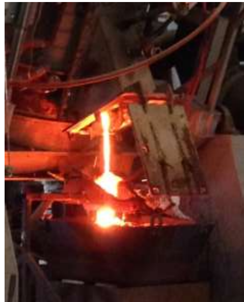
Figure 4. Pouring of hot slag
