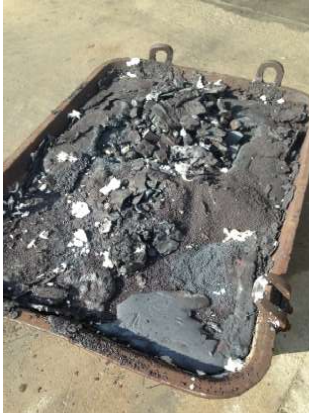
Figure 8. Collected total amount 235l slag in a 272l receptacle
