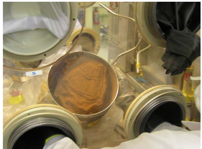
Figure 4: rust in 30-l can
