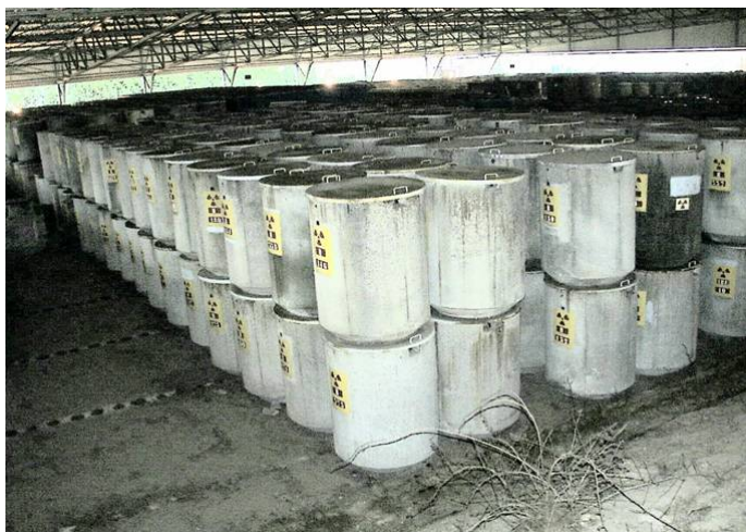
Fig. 1 (2003) : Overview of the concrete shielded containers
